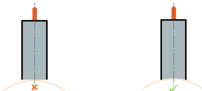
Fig. 1 – Improper (✗) and correct (✓) seating of a carbon brush contact face
